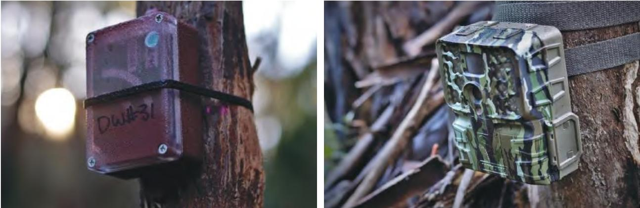
Figure 2: (Left) Camera Trap (Right) AudioMoth (an automated acoustic recording device) in waterproof case. (Photo: Darcy Whittaker)
